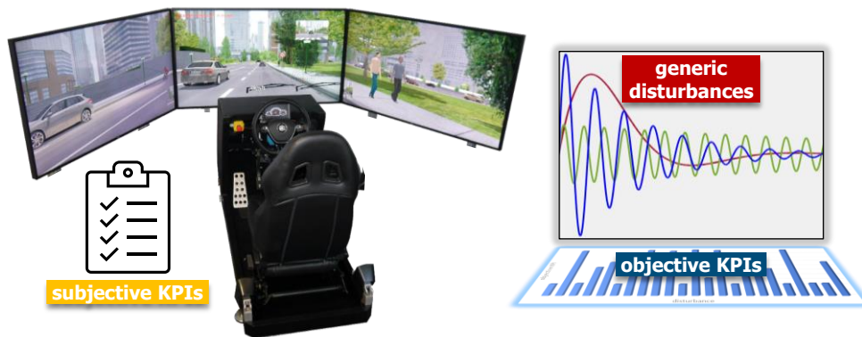
Fig. 3. Driving simulator tests with generic disturbances and objective KPIs by digital twin
